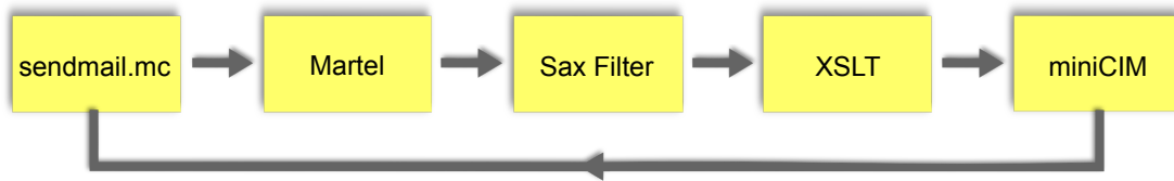
Figure 7.3: Process to transform the Sendmail configuration to miniCIM
