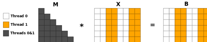
Figure 3: Example of the BLAS3 triangular solver with M replicated and X and B distributed by columns
