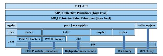
Figure 1. Overview of the MPJ Express design. MPJ, Message Passing in Java; JFS, Java Fast Sockets; IO, Input/Output; NIO, New IO; JNI, Java Native Interface; MX, Myrinet Express; MPI, Message-Passing Interface.
