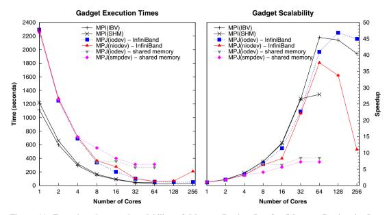
Figure 11. Execution times and scalability of Message-Passing Interface/Message Passing in Java (MPI/MPJ) Gadget on the Finis Terrae. IBV, InfiniBand Verbs; SHM, shared memory.
