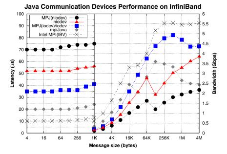
Figure 6. Message-passing point-to-point performance on InfiniBand (x86\_64 cluster). MPJ, Message Passing in Java; MPI(IBV), Message-Passing Interface (InfiniBand Verbs).
