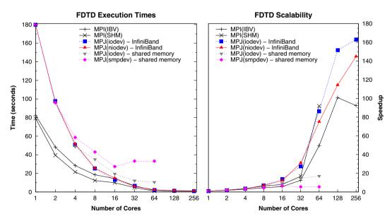
Figure 10. Execution times and scalability of Message-Passing Interface/Message Passing in Java finitedifference time-domain (MPI/MPJ FDTD) on the Finis Terrae. IBV, InfiniBand Verbs; SHM, shared memory.
