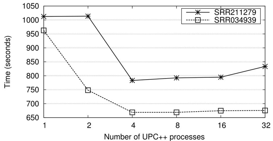
**Fig 4. Runtimes (seconds) of the single-end alignment using all the 64 cores of one node and varying the combinations of processes/threads (from one process with 64 threads to 32 processes with two threads each).**
