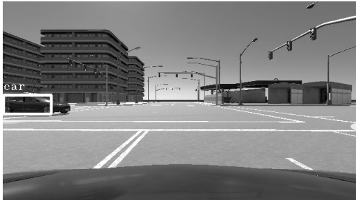
Fig. 1: Frame from the camera in the front bumper of the car simulated in CARLA. On the left side of the image, the other car is shown, surrounded by a box that indicates that YOLO identifies the object as a car.
