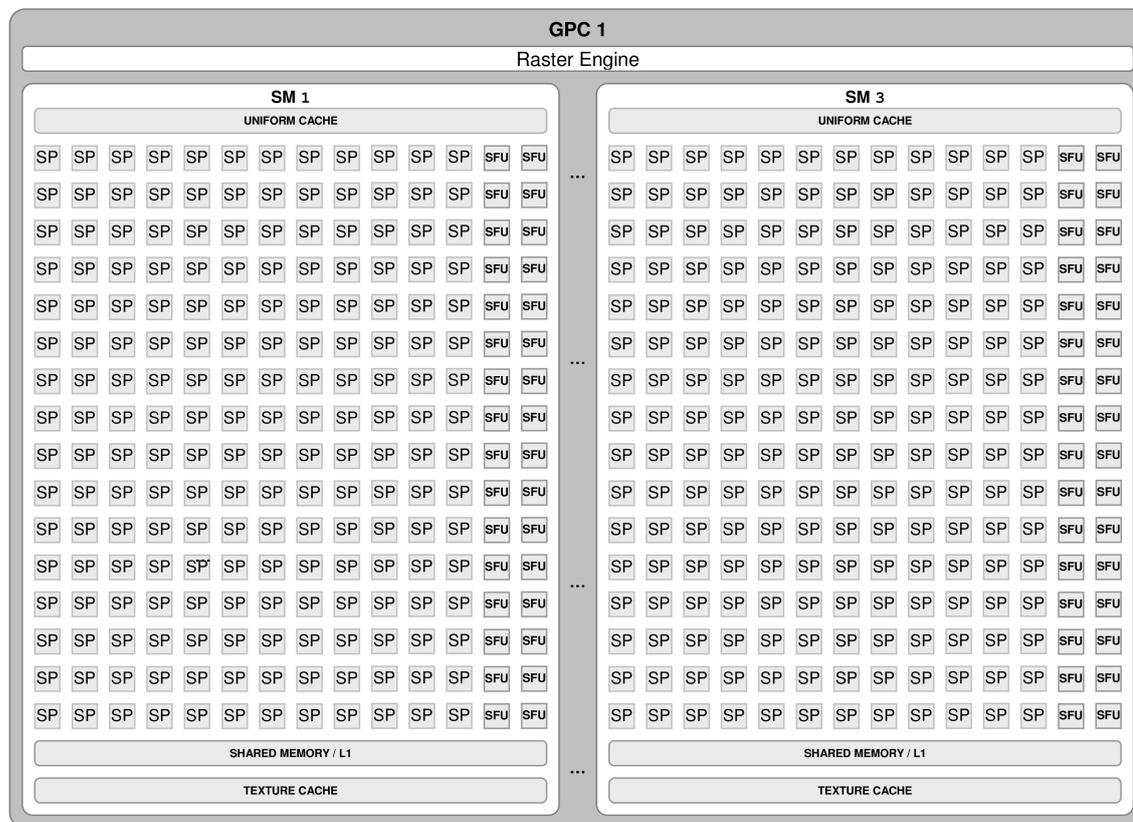
Figure 1.4: Kepler architecture used in the GeForce Titan
