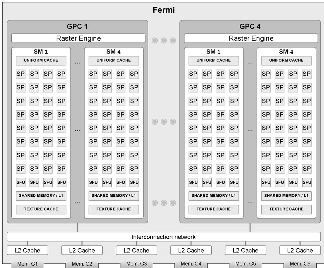
Figure 1.3: Fermi architecture used in the GeForce 480
