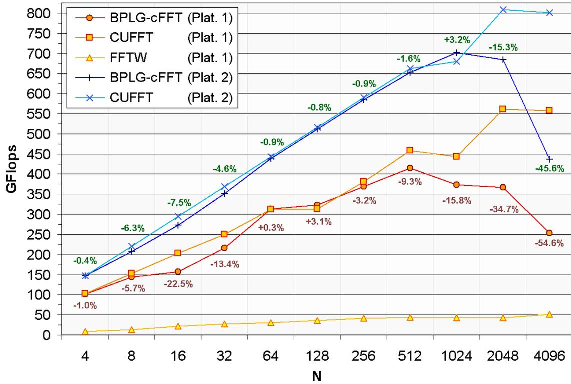
Figure 4.7: Algorithm performance for the complex FFT algorithm
