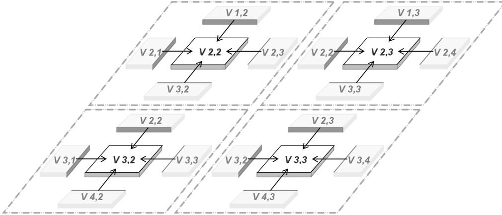
Figure 2.12: Recomputation-based solution on a multithreading system
