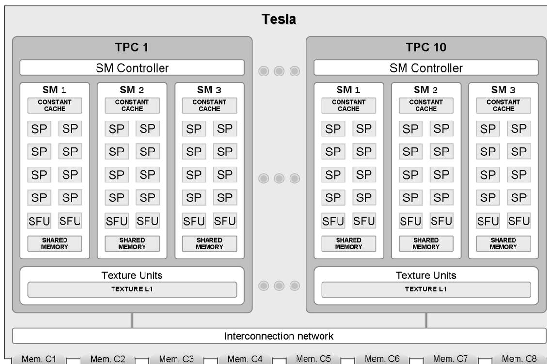
Figure 1.2: Tesla architecture used in the GeForce 280
