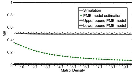
Figure 4.8: Miss rate measured and predicted following different strategies as a function of the matrix density for the sparse matrix-dense matrix product (IKJ), where  $M = N = H = 500$  in a cache of 64Kbytes with a line size of 64 bytes and associativity degree 4.
