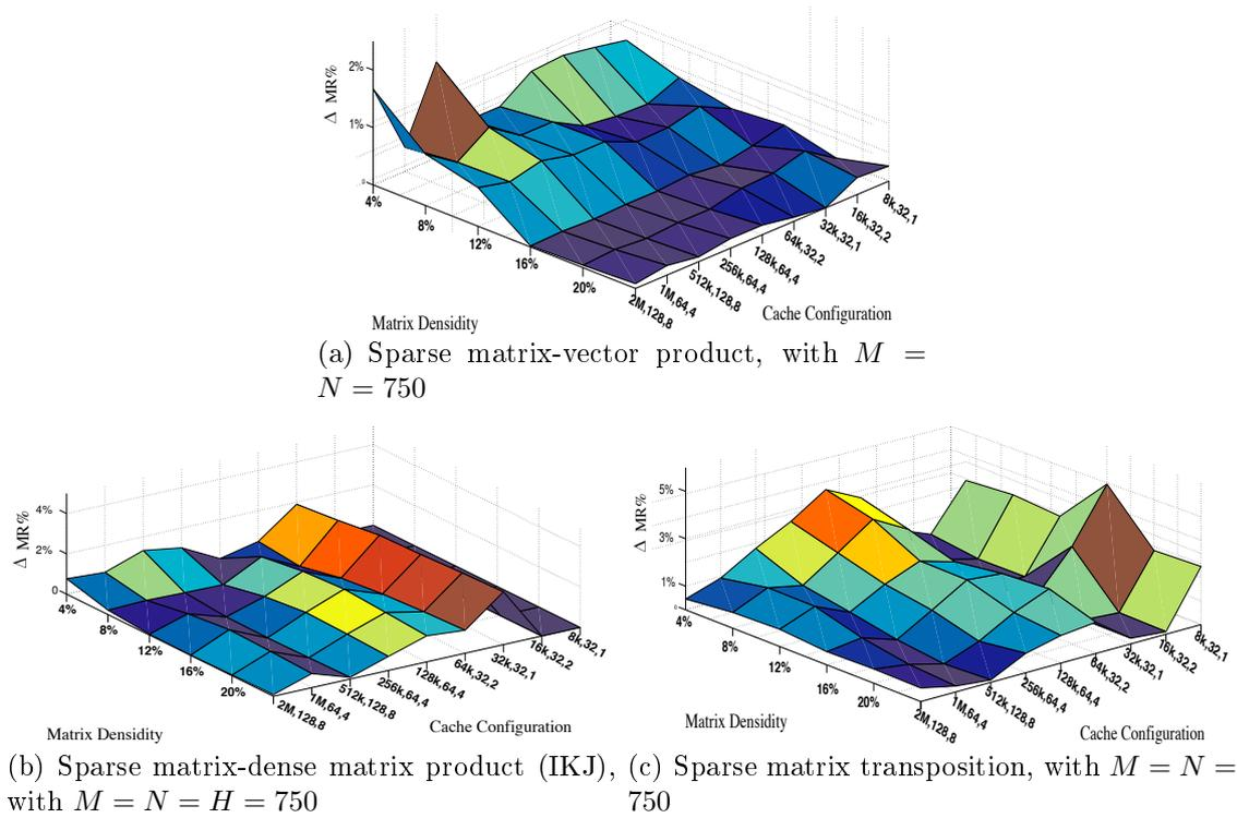
Figure 4.7:  $\Delta_{MR}$  as a function of the sparse matrix density and the cache configuration in different codes. Cache configurations are expressed as  $C_s, L_s, K$ , where  $C_s$  is the cache size in bytes,  $L_s$  is the line size in bytes and  $K$  is the associativity
