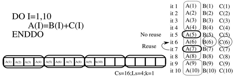
Figure 2.1: Reuse in a simple loop
