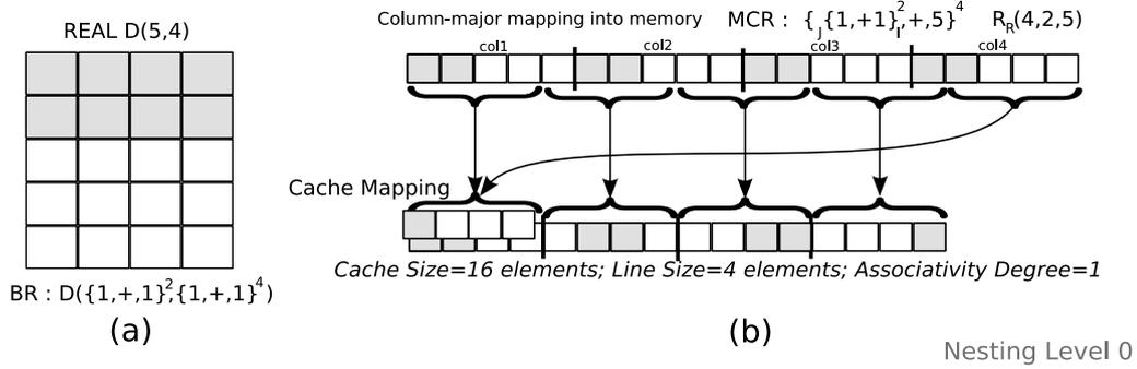
Figure 5.3: Matrix mapping in memory and in cache for reference  $D(I, J)$  of Figure 4.5 during 2 iterations of loop  $do_I$
