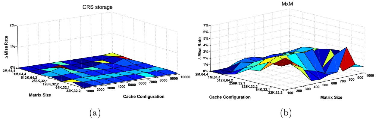
Figure 3.8: Surfaces representing the  $\Delta_{MR}$  evolution for different cache configurations and matrices sizes in the CRS storage and optimized matrix product codes. The cache configuration is denoted using the notation  $(C_s, L_s, k)$ .
