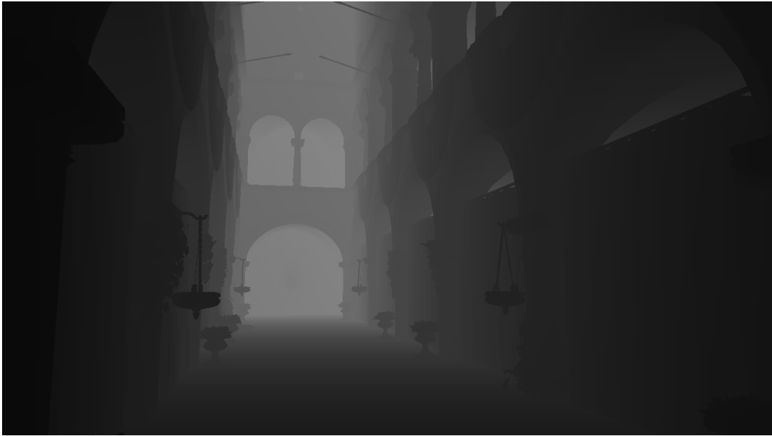
Figura 6.5: Depth Buffer o Z-Buffer, a mayor claridad, mayor profundidad
