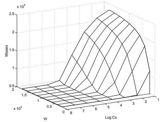
Figure 8: Number of misses during the sparse matrix-vector product for a sparse matrix  $20K \times 20K$  with  $N_{\text{NZ}} = 2M$  entries,  $L_S = 8$  and  $K = 4$  as a function of  $W$  and  $C_S$ .
