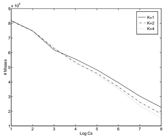
Figure 11: Number of misses during the transposition of a sparse matrix  $20K \times 20K$  matrix with  $2M$  entries and  $W = 8000$  as a function of the cache size with  $L_S = 8$  for different associativities.
