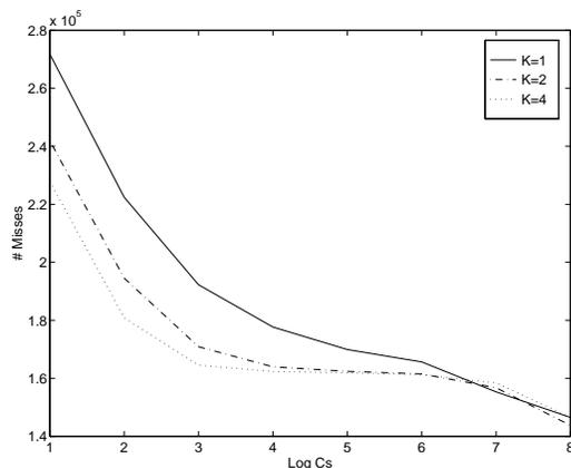
Figure 13: Number of misses during the transposition of a sparse matrix  $5K \times 5K$  matrix with 125K entries and  $W = 200$  as a function of the cache size with  $L_S = 4$  for different associativities.
